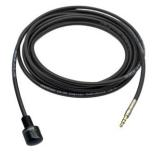
The 3.5mm TRS plug can be connected directly to a standard 3.5mm mic jack that supplies plug-in power (PIP) (2.4V, min.  $400\mu$ A). It is wired dual mono: tip and ring (output), sleeve (ground). The outside diameter is 5.5mm.
