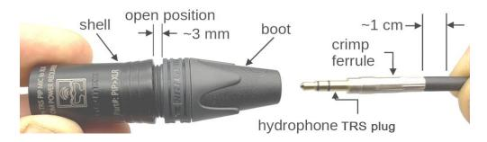
The boot compresses a plastic chuck that holds the hydrophone TRS plug in place. When open, you will see a gap of approximately 3mm between the boot and shell of the XLR connector. Hold the hydrophone cable approximately 1 cm behind the crimp ferrule on the TRS plug.
