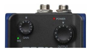
You can adjust the input gain by turning the gain knob on the XLR-to-USB sound card (see figure above). To account for this gain adjustment, you will have to update the "Probe" switch position (see figure below) accordingly in Multi-Instrument's toolbar.
