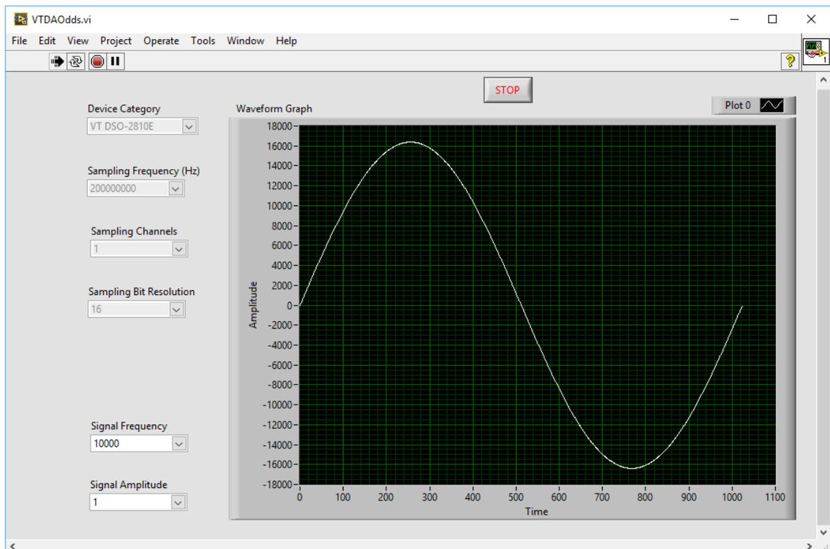
vtDAOdds.vi is a sample VI for Labview programming using vtDAO interfaces. vtDAO interface wrapper: vtDAOLV.dll, is called using Labview Call Library function node. It is basically a signal generator VI with adjustable sampling parameters, signal frequency and signal amplitude. To keep the VI simple, these parameters cannot be changed on-the-fly.
