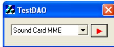
TestDAO is a sample DAO back-end program. It demonstrates how to use the vtDAO interfaces to perform data output. There are one Start/Stop button for starting/stopping DAO and one combo box for selecting vtDAO interface DLLs. All the DAO parameters are set inside the software codes. No GUIs (Graphical User Interface) are provided for changing these parameters for simplicity purpose. Both DDS and streaming modes are demonstrated in this program.
