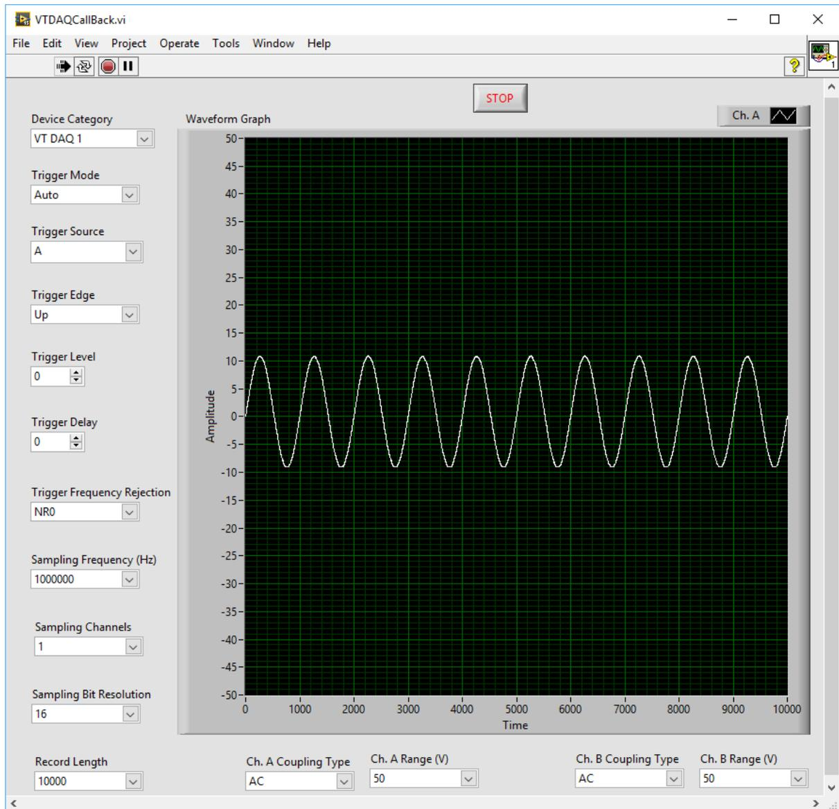
vtDAQCallBack.vi is a sample VI for Labview programming using vtDAQ interfaces. VtDAQ interface wrapper: vtDAQLV.dll, is called using Labview Call Library function node. It is basically an oscilloscope VI with adjustable sampling and triggering parameters. To keep the VI simple, these parameters cannot be changed on-the-fly.
