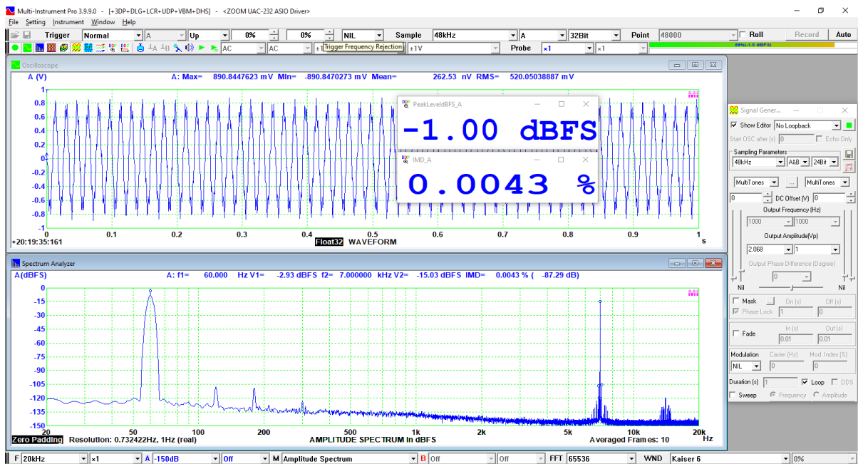
SMPT E IMD of XLR input measured at -1 dBFS (digital gain = 0 dB)
