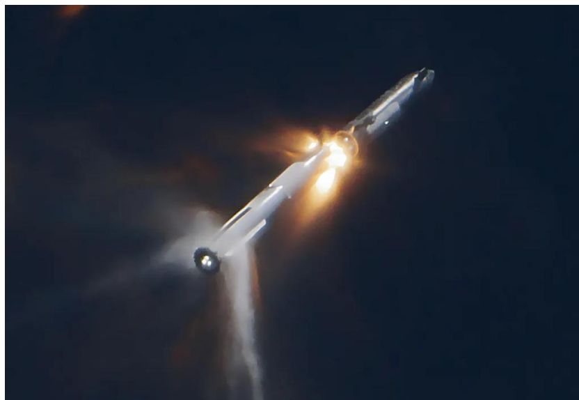
Rocket Hot-stage Separation
