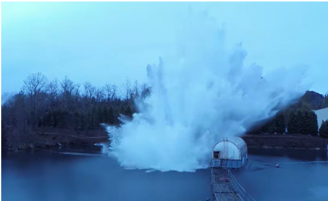
A Barge Shock Test
