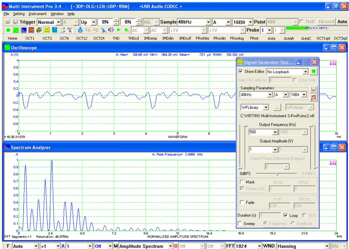
Measured 500Hz truncated sine wave from a computer speaker with its polarity inverted
