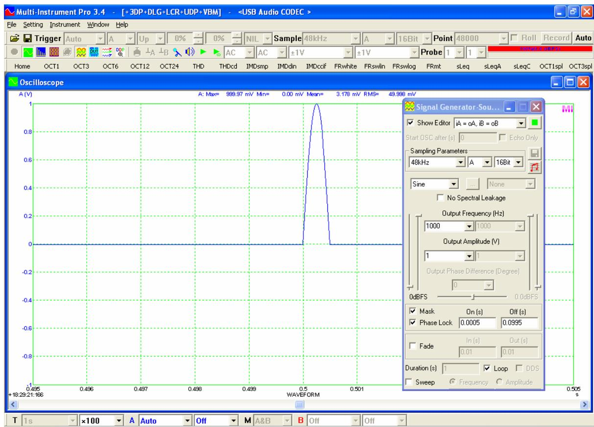
Ideal 0.5 ms 1 kHz half sine burst at a repetition rate of 100 ms
