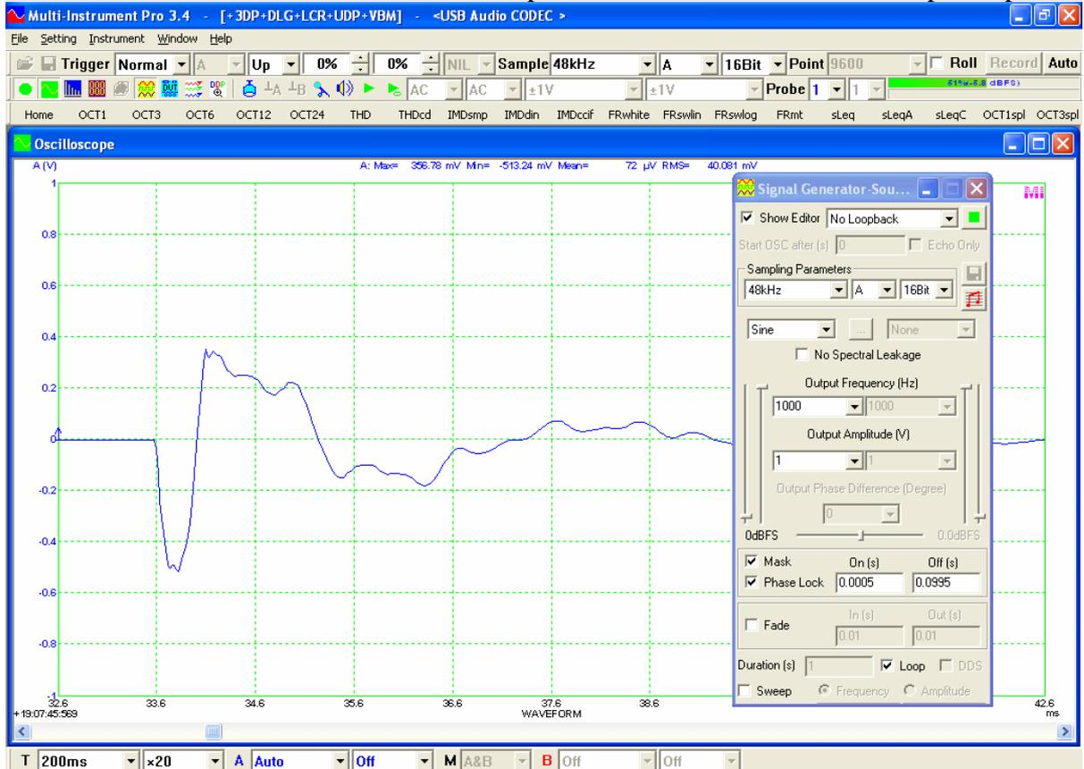
Measured 0.5 ms 1 kHz half sine burst at a repetition rate of 100 ms from a computer speaker with its polarity inverted
