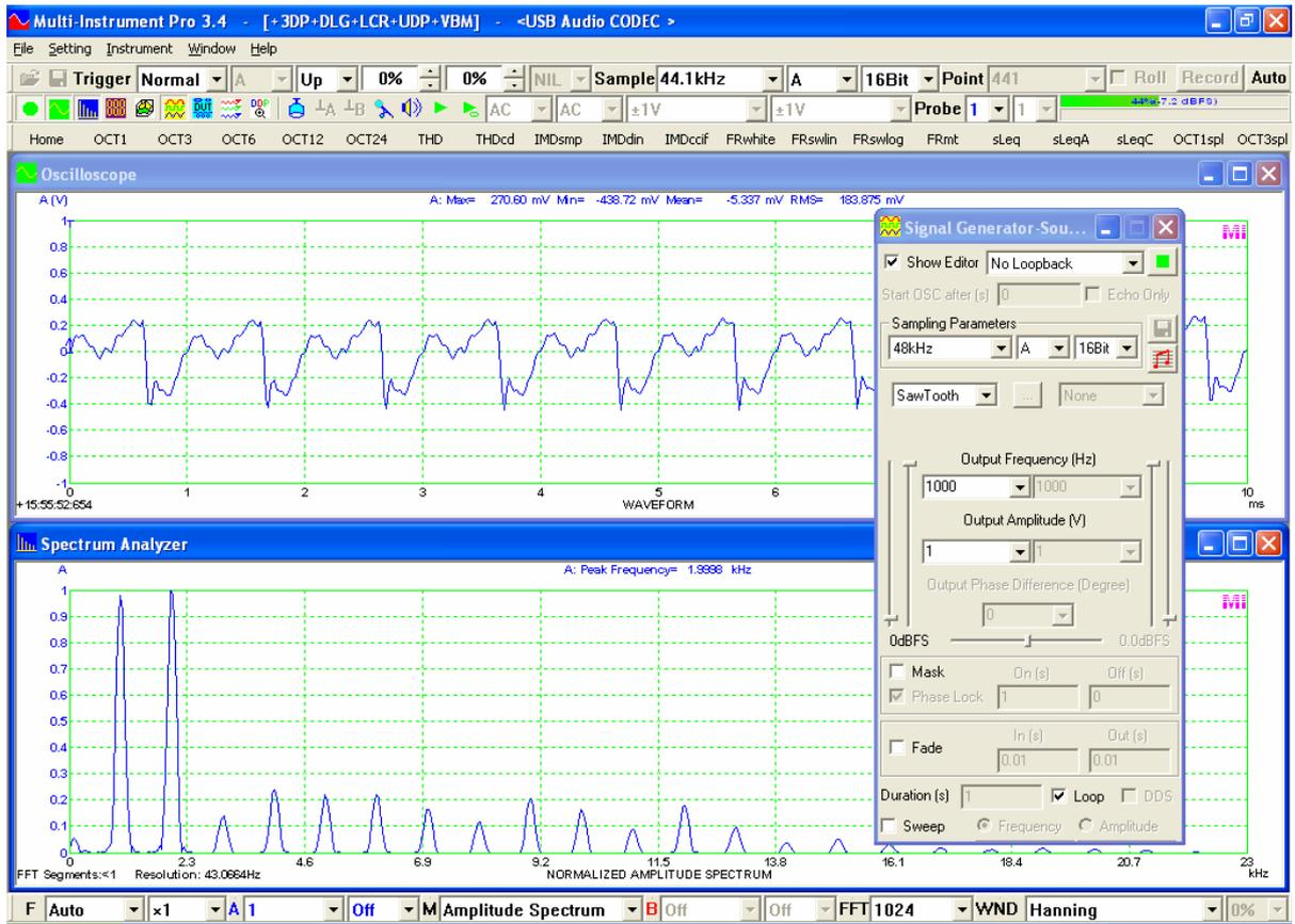
Measured 1kHz sawtooth wave from a computer speaker
