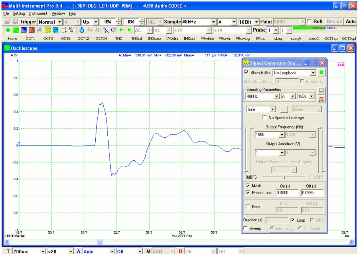
Measured 0.5 ms 1 kHz half sine burst at a repetition rate of 100 ms from a computer speaker
