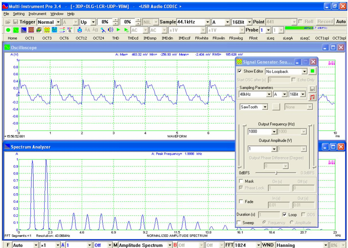
Measured 1kHz sawtooth wave from a computer speaker with its polarity inverted
