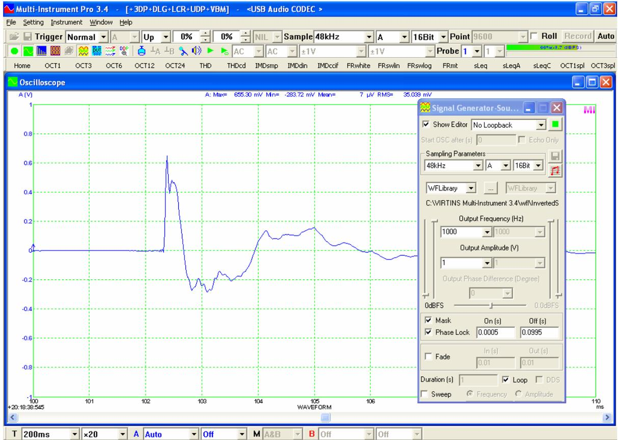
Measured 0.5 ms 1 kHz half inverted sawtooth burst at a repetition rate of 100 ms from a computer speaker
