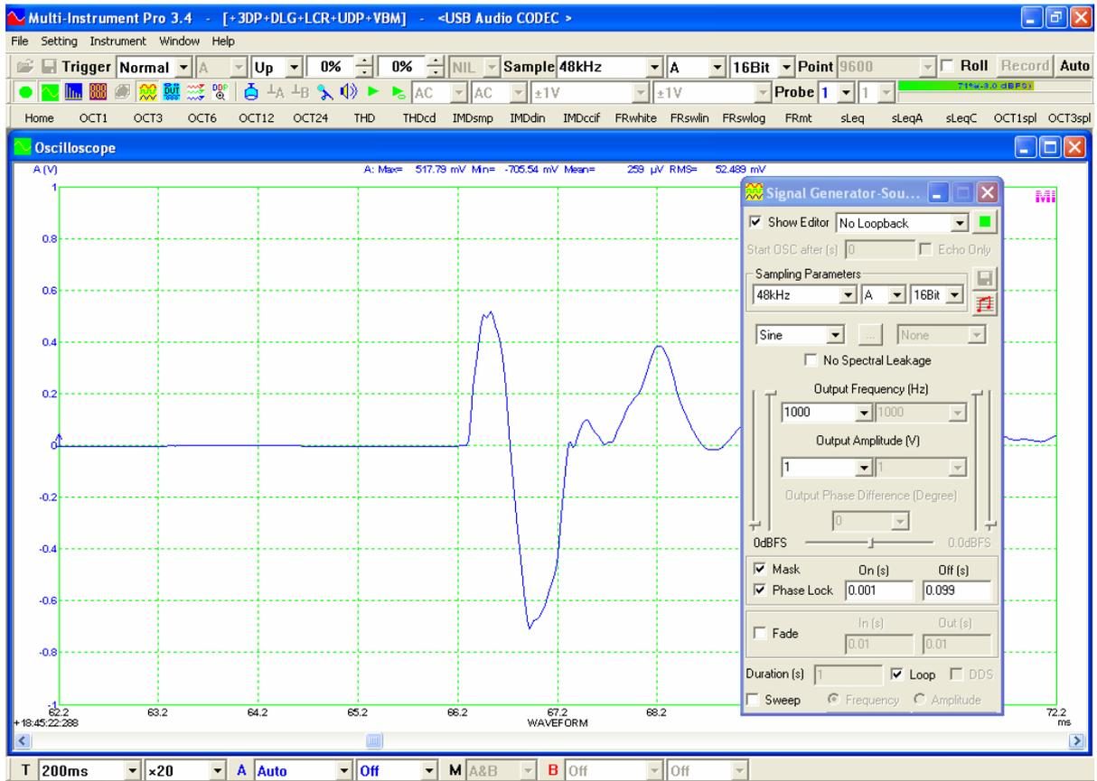
Measured 1 ms 1 kHz sine burst at a repetition rate of 100 ms from a computer speaker
