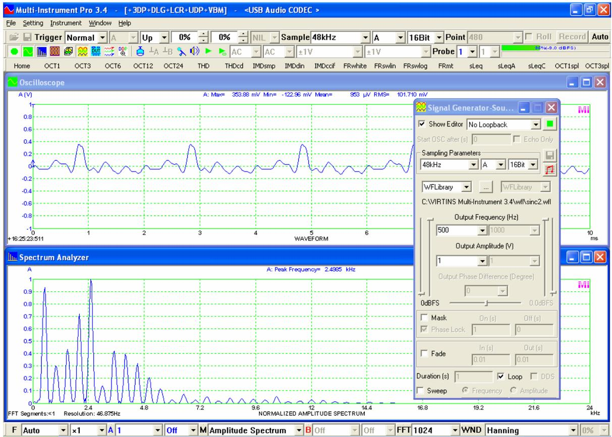
Measured 500Hz truncated sine wave from a computer speaker
