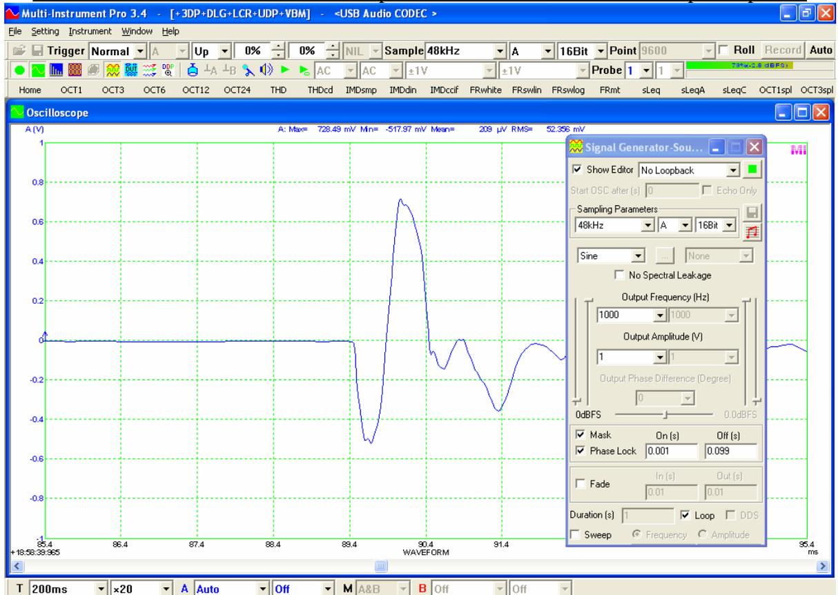
Measured 1 ms 1 kHz sine burst at a repetition rate of 100 ms from a computer speaker with its polarity inverted
