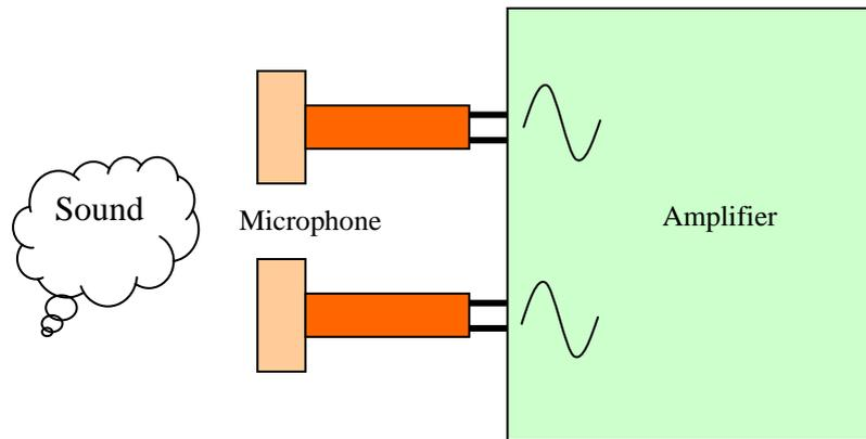
Relative Polarity Maintained in Sound Recording
