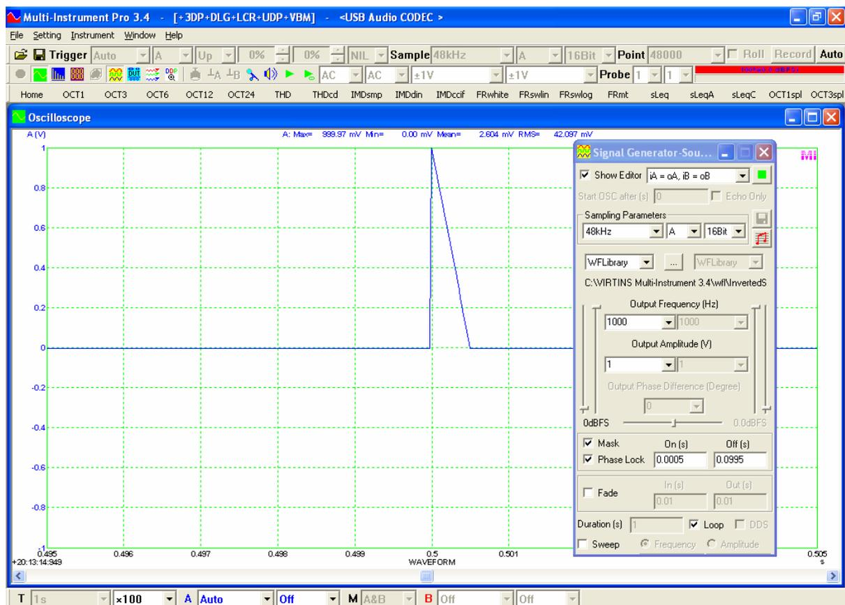
Ideal 0.5 ms 1 kHz half inverted sawtooth burst at a repetition rate of 100 ms
