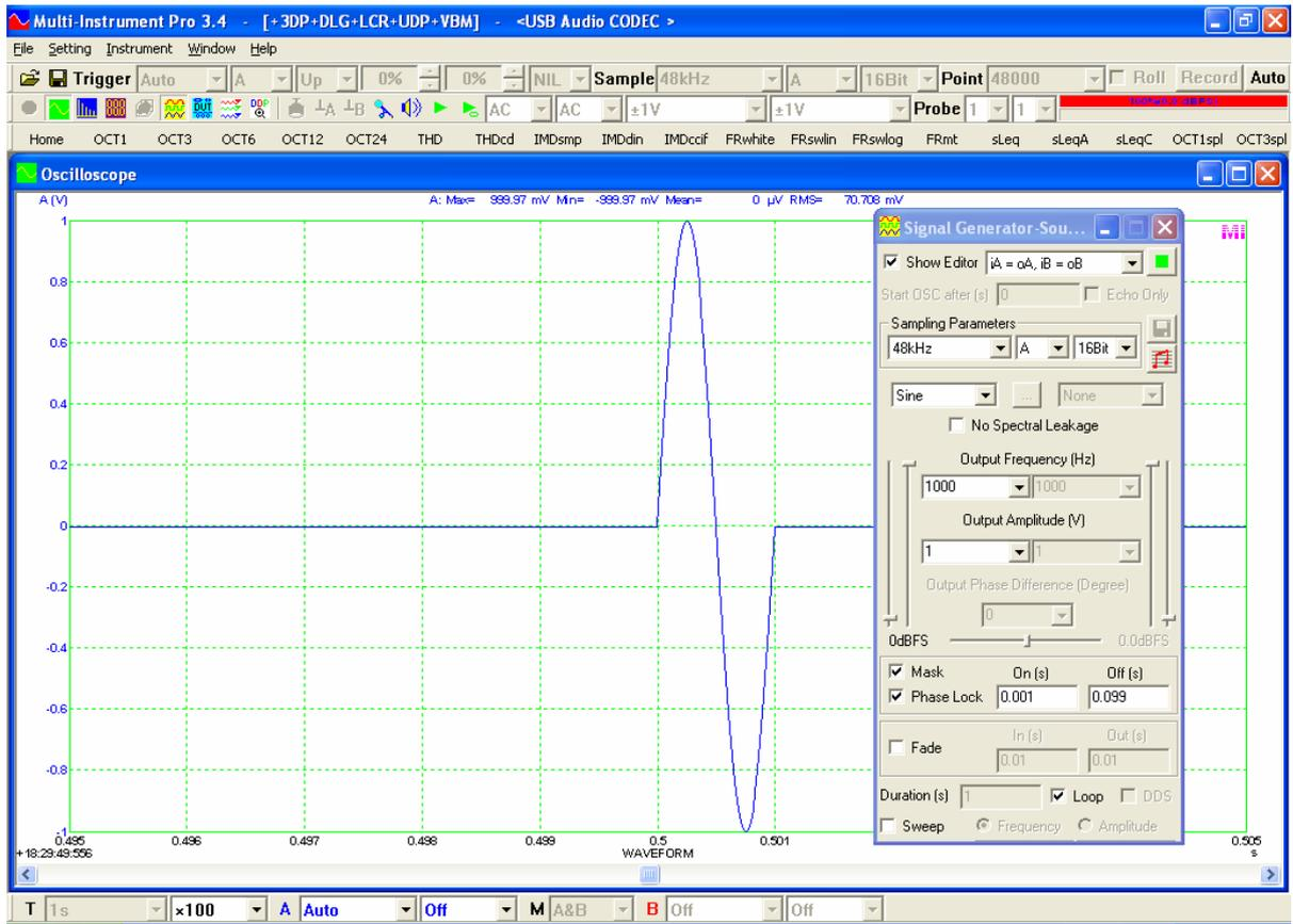
Ideal 1 ms 1 kHz sine burst at a repetition rate of 100 ms
