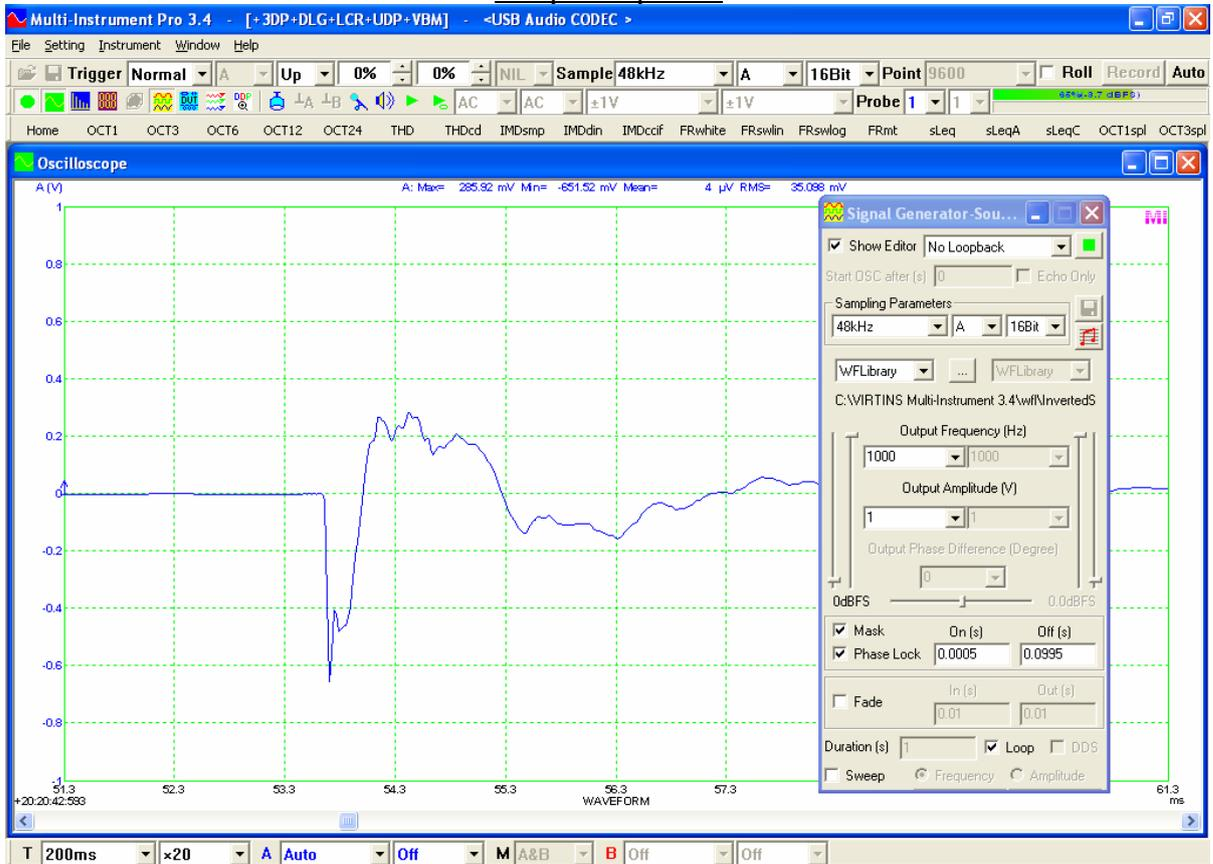
Measured 0.5 ms 1 kHz half inverted sawtooth burst at a repetition rate of 100 ms from a computer speaker with its polarity inverted
