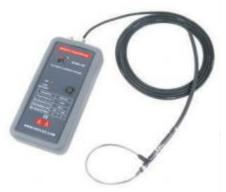
OEM Rogowski coil on request. Coil circumference from 120mm to 1000mm for AC current, Max. bandwidth 15 MHz, Max. current 350 kA. Flexible coil makes measurement more flexible.
